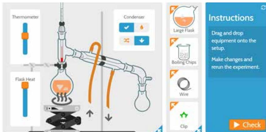
How do you practise an experiment before the lab starts? The DLM's online simulations allow you to interact with equipments you will encounter in the lab. If you're unsure how to set up a distillation apparatus, you can have a go online and get feedback to lead you through the process. To better understand IR spectroscopy, you can interactively change the atoms on each end of a chemical bond and see how this influences the frequency at which the bond vibrates.
